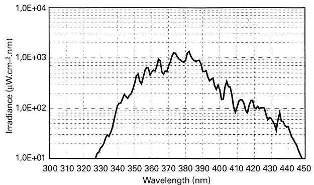
Figure 1. Emission spectrum of Jetsun 55 UVA lamp.
