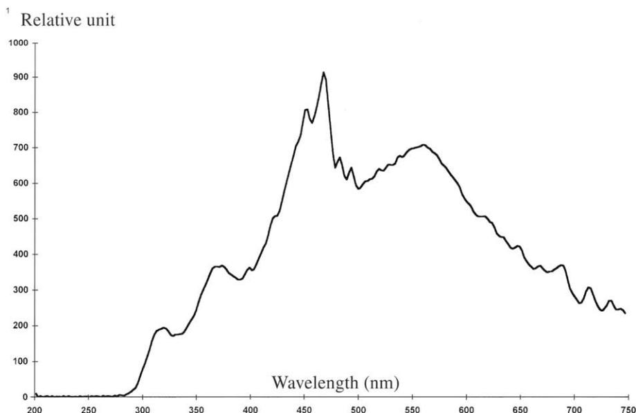
Fig. 1. Total emission spectrum of Dermolum UM-W lamp with WG-305 filter.
